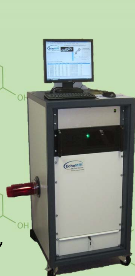
Fig 2. Echo MRI: measures fat and water content.
