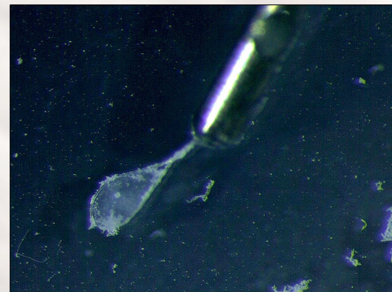
Figure 5: Demonstration of ice crystal formation of a water droplet in a Cryoloop plunged into LN 2
