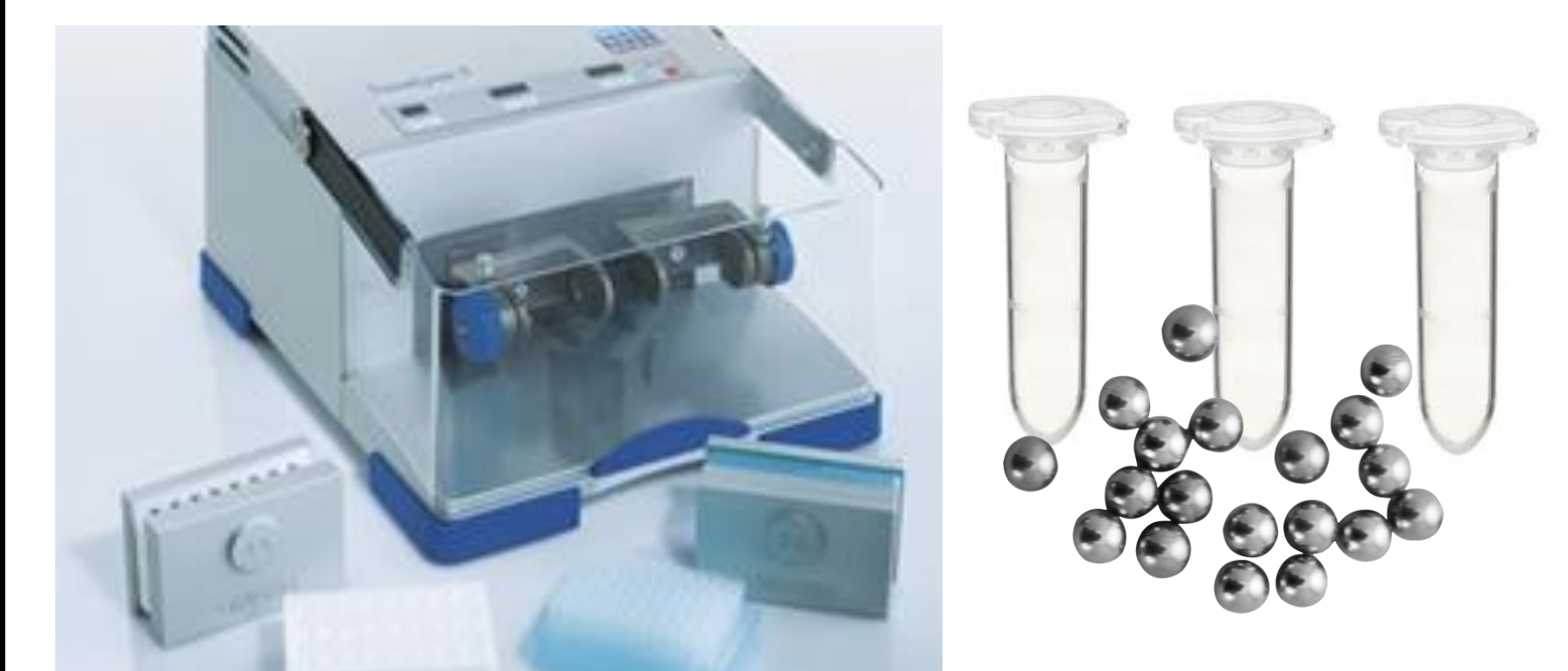
Figure 6: TissueLyser II machine, tubes and steel beads used to homogenize tick samples.
