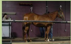
A: Sensor placed on poll to measure vertical head acceleration 3: Sensor placed on cranial side of pastern used as stride marker C: Sensor placed between the tubera sacrale measuring vertical pelvic acceleration
